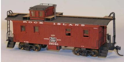
an inner body, peel and stick the sides, ends, windows, trim, etc. which is all cut out of adhesive backed wood. Kit-bash the included Athearn caboose frame with the included pre-cut parts. Form and install grab irons from the included brass wire. Paint and letter.
