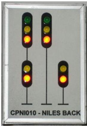
Fig. 3 A repeater in service. Note the trim made out of Evergreen 294 angle cut with a NWSL chopper. The red lights are all lit indicating that no route has been cleared through the interlocking.
