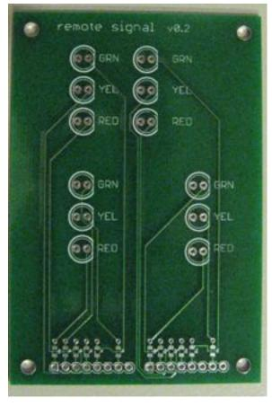
Fig. 1 The front side of an un-stuffed circuit board.
