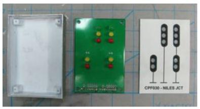
Fig. 2 The styrene box, assembled circuit board, and laser cut and engraved face plate.
