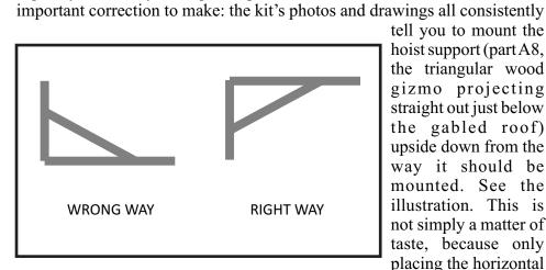
tell you to mount the hoist support (part A8, the triangular wood gizmo projecting straight out just below the gabled roof) upside down from the way it should be mounted. See the illustration. This is not simply a matter of taste, because only placing the horizontal
