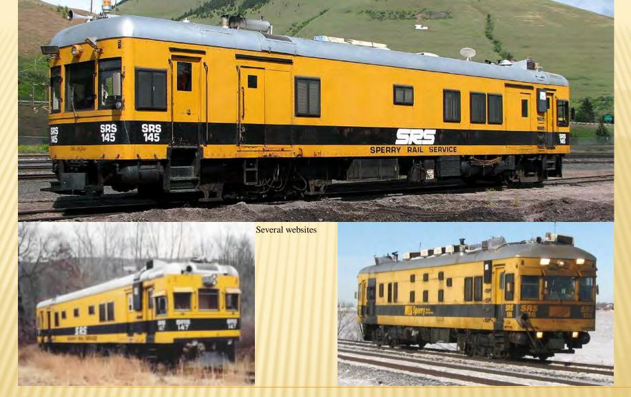
Sperry Rail Service has provided rail inspection services on contract to the railroads since 1928. The process detects flaws in rails, then mark the spot and reports to the railroad.
