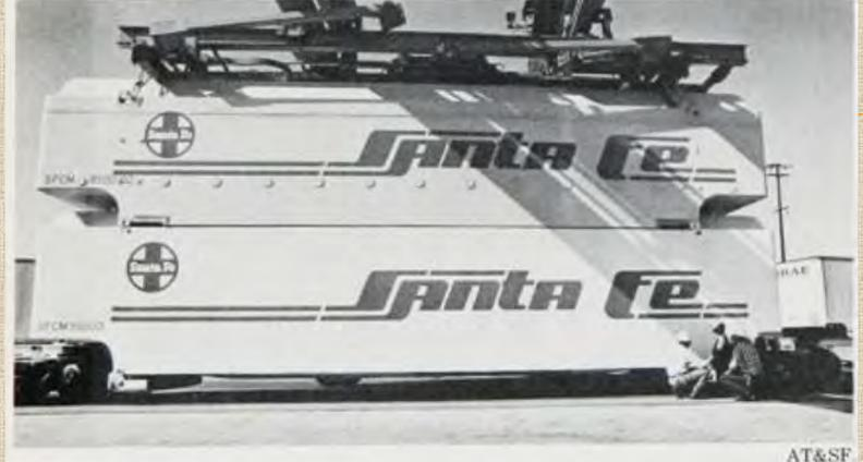
EACH of these new double-stacked intermodal containers developed by Santa Fe can accommodate up to 55 tons of bulk lading, palletized packaged goods, or liquids; are made of fiberglass or aluminum; and ride on the railroad's Fuel-Foiler articulated cars.
