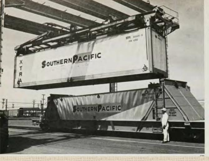
PIGGYBACK COFC: Southern Pacific is testing a flat car that will carry two stacked 40-foot containers. Built by ACF, No. 513300 is 18½ feet high over the load.
