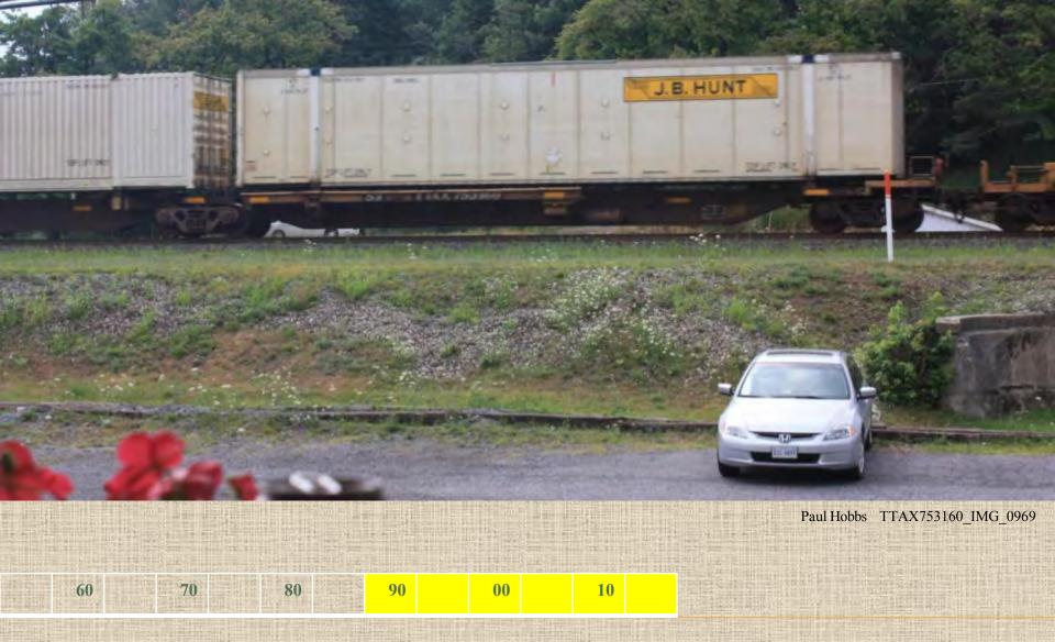
TTAX 753160 on Norfolk Southern train at Cresson, Pennsylvania in July 2011 Multiple platform spine car for up to 53-foot trailer or container.
