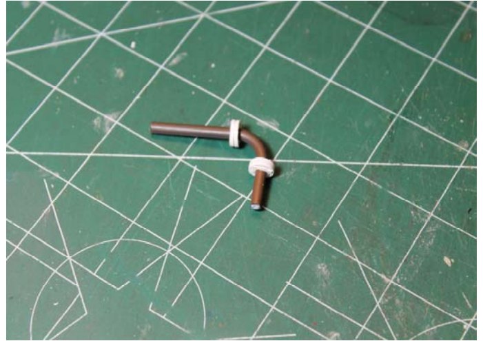
The Round Tops of the Wall Anchors Are Sliced off and Slid Onto the Sprue To Form a Flanged Elbow.
