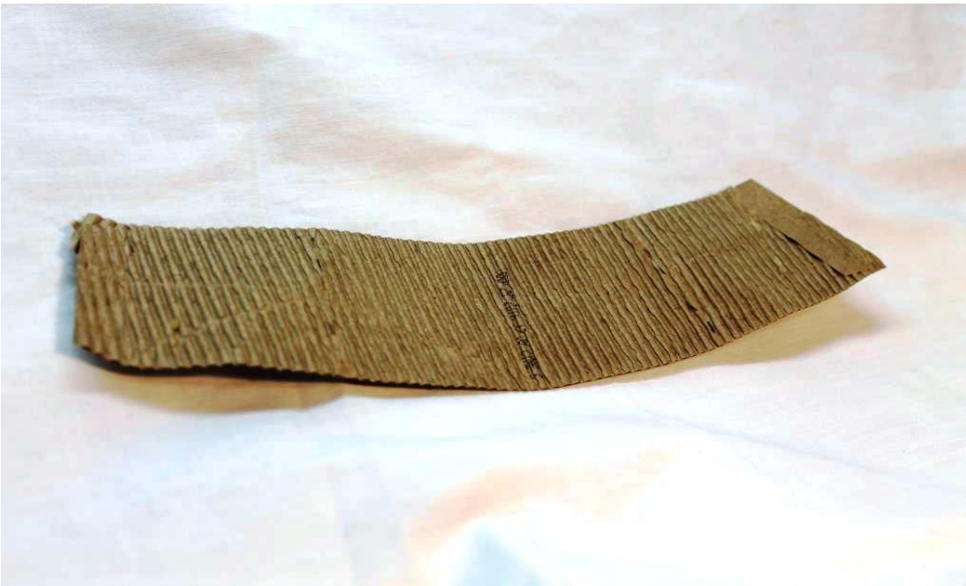
Starbuck's® coffee gripper folder out makes fluted tile material
