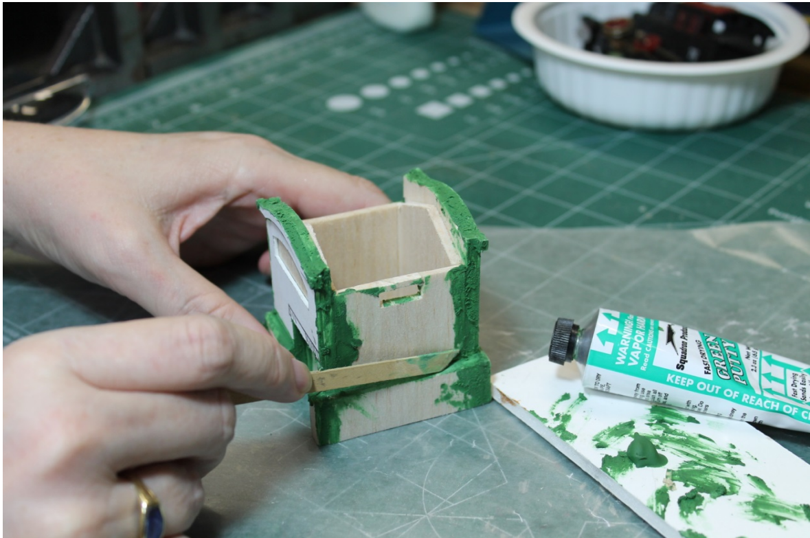
Putty is Used to Fill and Shape the Exterior Walls and Door & Window Openings.
