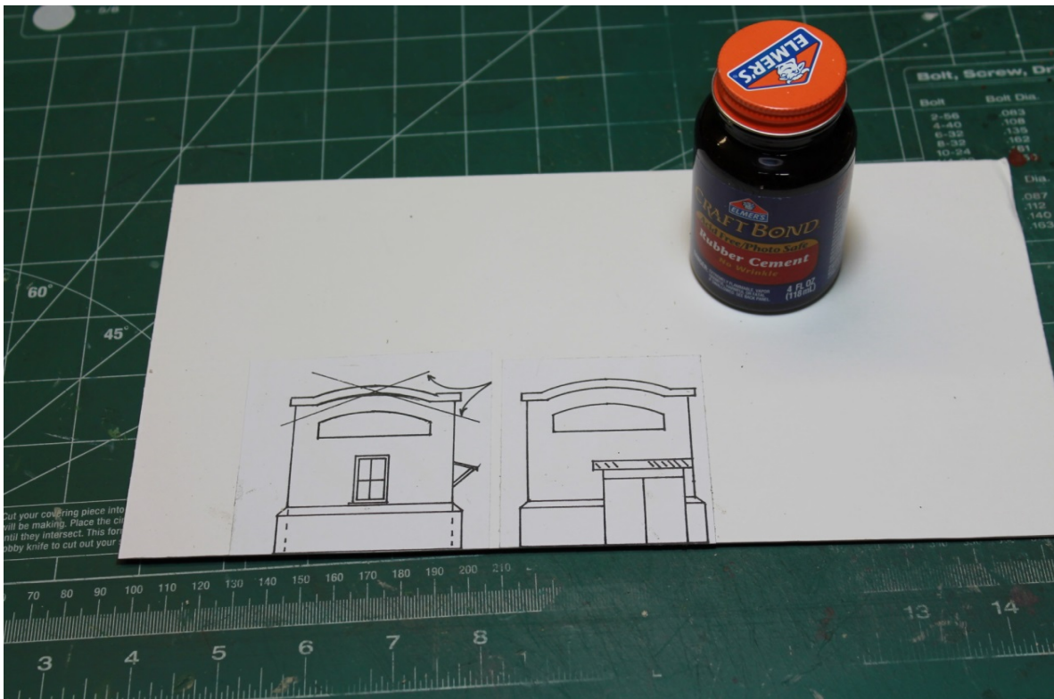
Scale Drawing is Laminated to Matt Board with Rubber Cement.
