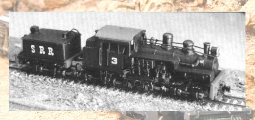
THREE TRUCK SHAY BUILT BY ROGER HORD (AUS) TO RUN ON .256" (6.50 MM) GAUGE TRACK
