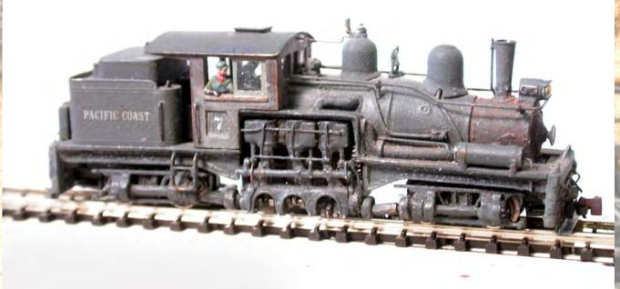
TWO TRUCK SHAY WITH OPERATING CRANK- AND DRIVE-SHAFTS SCRATCH-BUILT BY AUTHOR DURING 1980'S, TO RUN ON .256" (6.50 MM) GAUGE TRACK
