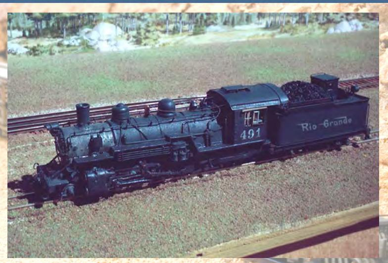
K-37 #491 SCRATCH-BUILT BY AUTHOR DURING 1980'S, TO RUN ON .256" (6.50 MM) GAUGE TRACK (was used as pattern for RLW kit)
