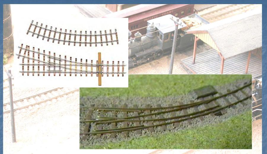
Nickel-Silver rail soldered to printed-circuit-board (PC board) ties in a jig, then transferred to the layout.
