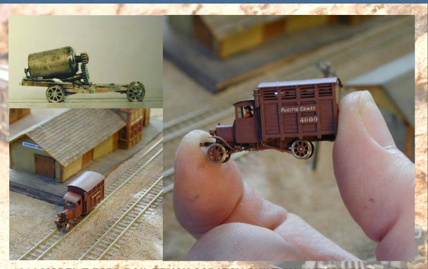
1914 MODEL T FORD RAIL TRUCK SCRATCH-BUILT BY AUTHOR TO RUN ON .256" (6.50 MM) GAUGE TRACK, USING "PAGER" MOTOR
